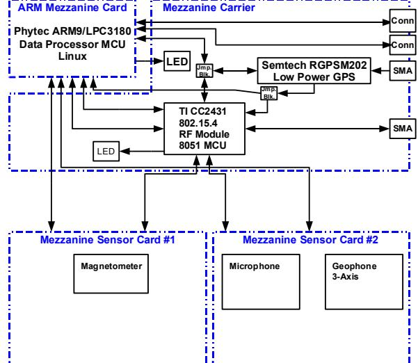
Fig. 3. Proposed modular node architecture
