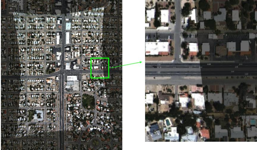
Figure 1. This shows a frame of imagery taken from the helicopter transparently superimposed over a region of the same image acquired from GoogleMaps. The region in the green box on the left is shown zoomed in on in the image on right. The curved boundaries of the image are due to the radial distortion correction and registration processes.
