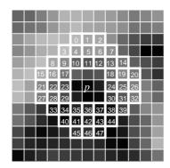
$\label{eq:Fig.6} \mbox{Fig. 6}$  Positions of offsets used in the FAST-ER detector.
