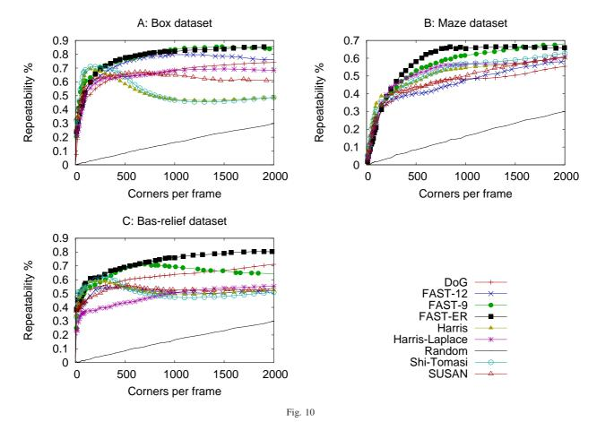
A, B, C: Repeatability results for the repeatability dataset as the number of features per frame is varied. D: Key for this figure, Figure 11 and Figure 9. For FAST and SUSAN, the number of features can not be chosen arbitrarily; the closest approximation to 500 features in each frame is used.
