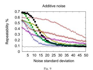
Repeatability results for the bas-relief data set (at 500 features per frame) as the amount of Gaussian noise added to the images is varied. See Figure 10 for the key.
